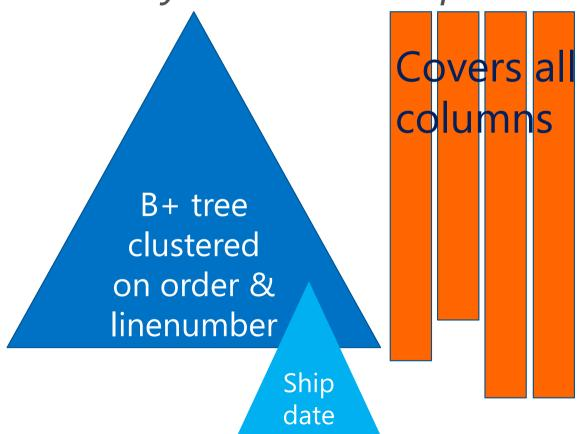
Heap file base table Secondary Columnstore Secondary B+tree on ship date
